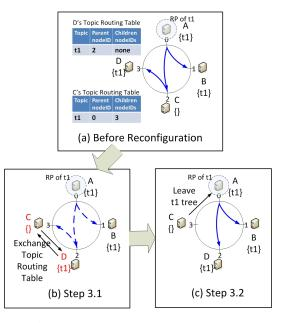
Figure 4: An example of the step 3 of the reconfiguration protocol. Solid lines in (a) shows topic t1's tree before reconfiguration. Broker "C" and "D" are reconfigured. Dashed lines in (b) shows the reconstructed tree after "C" and "D" exchange their data in step3.1. Solid lines in (c) shows the repaired topic routing tree after step 3.2.
