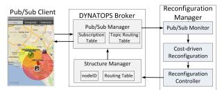
Figure 3: DYNATOPS Broker System Architecture
